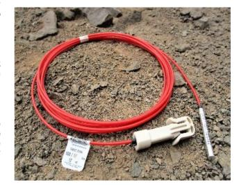
• "Mushroom-type" plastic connector: This is a plastic block, specially designed for facilitating connection and ensuring contact between the Fanel Shock Tube and the Surface Detonator, allowing the assembly of up to 6 shock tubes.
