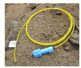
• "Mushroom-type" plastic connector: It is a plastic block specially designed to facilitate the connection and ensure contact between the delay detonator and the Fanel Shock Tubes. This element allows the assembly of several shock tubes.
