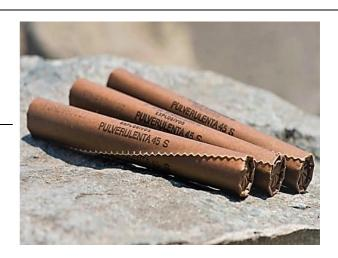
This DYNAMITE is used in all types of blasting operations in surface mining, underground mining, and civil works, being successfully employed in soft to intermediate rocks. Due to its low velocity of detonation and good sensitivity, it can be used in controlled blasting where spacers are employed to reduce the charge concentration. It is not recommended for use as a primer for nitro-carbonitrates (ANFO).
